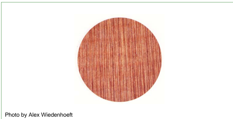
FIGURE F-2 Example of Araucaria araucana (Monkey puzzle tree) Wood Cross Section
